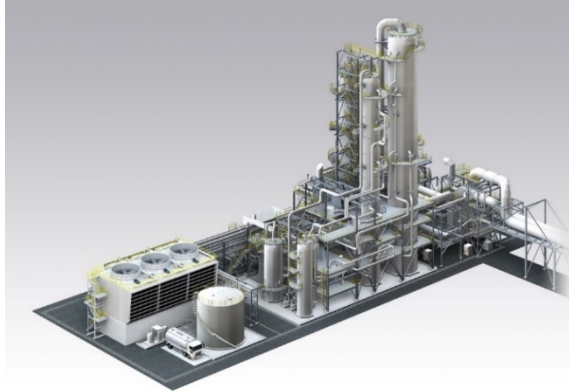
CO2 capture demonstration plant (under construction) Capture capacity: 500 tons/day
